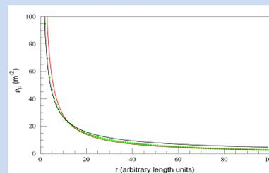
Figure 3. The  $\rho_\mu$  as a function of distance from the core of the air shower. The green circles are an evaluation of equation 6. The red line is proportional to  $r^{-1}$ . The black line is proportional to  $r^{-0.75}$ . At large distances from the core  $\rho_\mu \propto r^{-1}$ .
