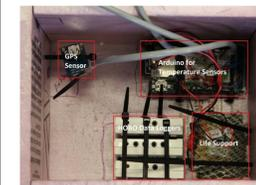
7. Picture of payload box with components.
