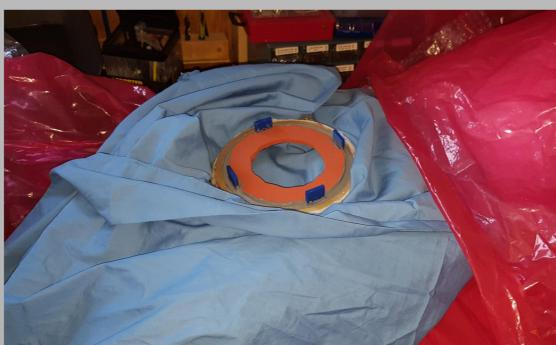
Figure 1: Process of sealing valve base into balloon apex
