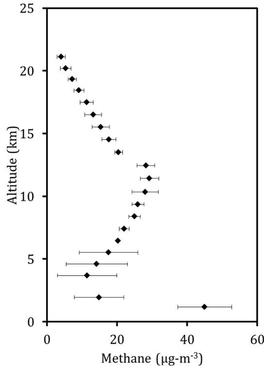
**Fig. 3 Methane profile measured with balloon borne MQ-2 detector. This is an average of four flights.**
