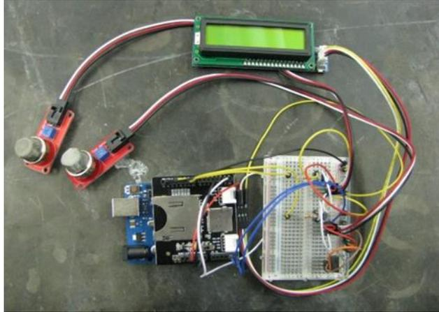
**Fig. 2 Arduino system with methane sensors. A SD card module is also shown which stores flight data. The LCD screen shown is used only during launch to make sure accurate data is collected.**
