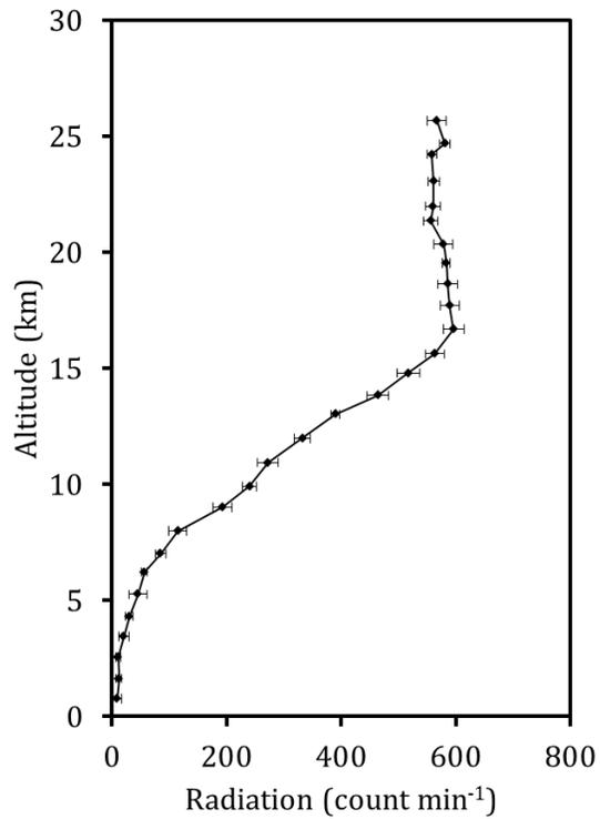
**Fig. 4 Methane profile measured with balloon borne MQ-2 detector. This is an average of four flights.**
