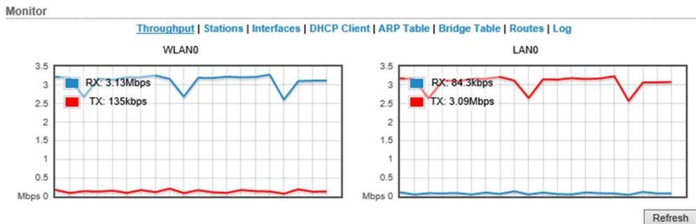
**Fig. 7 Receive and transmit data rates for streaming video from four webcams**
