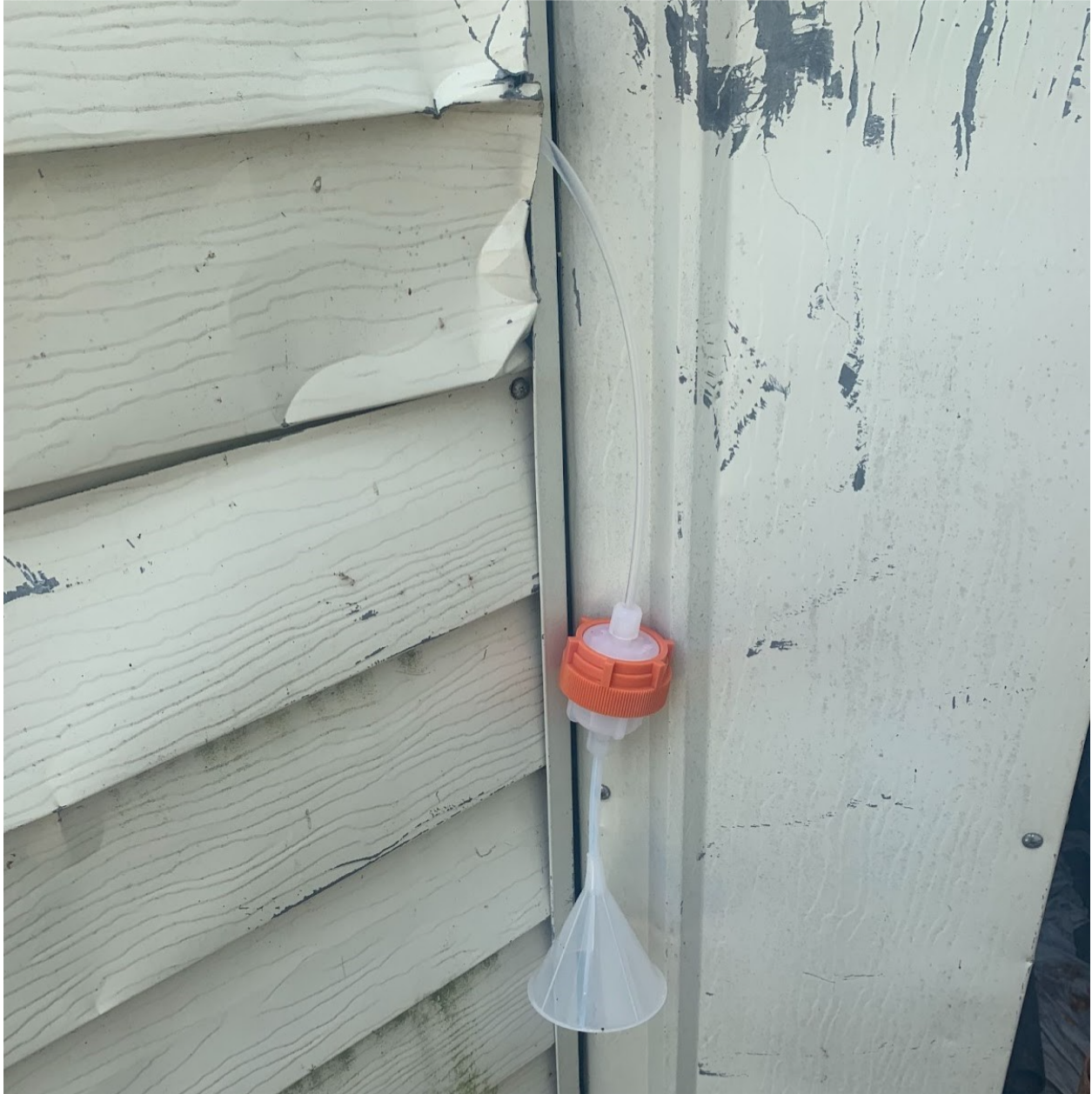
Figure 6. Filtered air tube installed in an outdoor shed at the PNNM site. The connected ozone monitor was located within the outdoor shed.
