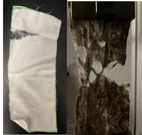
Figure 1. A fresh strip, left, tearing at one point versus a strip left in soil for five weeks, right, showing multiple point of weakness due to colonies of microbial decomposition.
