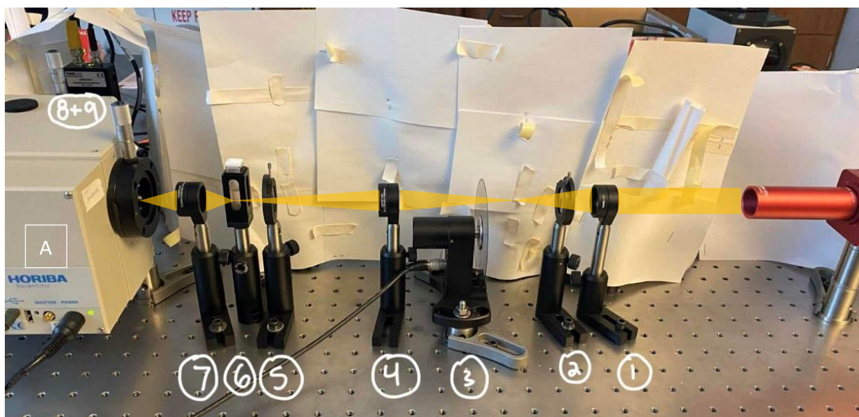
Figure 8. Side view of instrument. The red column is the tungsten light source, 25 mm biconvex lens (1), iris (2), oscillator (3), 50 mm biconvex lens (4), iris (5), cuvette holder (6), and 35 mm plano-convex lens (7). The SLS202L(M), Stabilized Tungsten light sources was used from Thor Labs. The settings on Lock-In Amplifier used were 2 x 1 mV.
