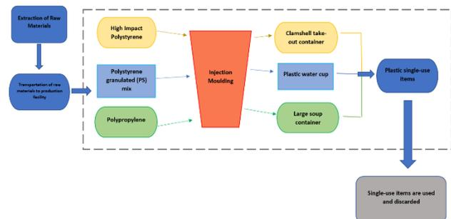
**Figure 1.** Process Flow Diagram for all plastic materials in this study. Exchanges (shapes) within the
