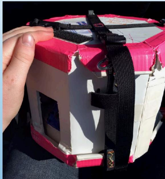
Fig. 4: Our payload after recovery. The camera is visible through a hole in the side of the payload box.
