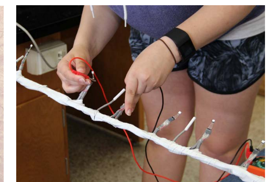
8. Checking continuity of installed sensors on wake arm bus.
