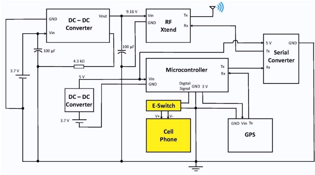
**Fig. 2 Block diagram of a dual-modal tracking payload.**
