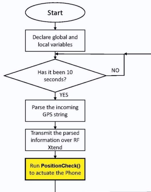
**Fig. 3 Overall flow chart for the operation.**
