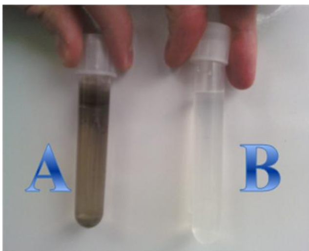
Figure 4.1: Auto-Decomposition of Dopamine. After 24 hrs dopamine visibly polymerizes in liquid LS media (A), however, acetylated dopamine remains unchanged (B).
