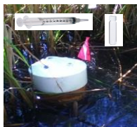
Figure 1.3: Example of capped chamber and gas collection tools, pictured here is a Typha control plot. Photo credit: Olivia Johnson.
