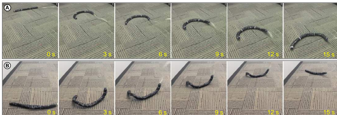
Figure 7.13: The SRS pose progression for (A) planar and (B) spatial rolling gaits at 3 \text{ bar} - 0.50 \text{ Hz} .
