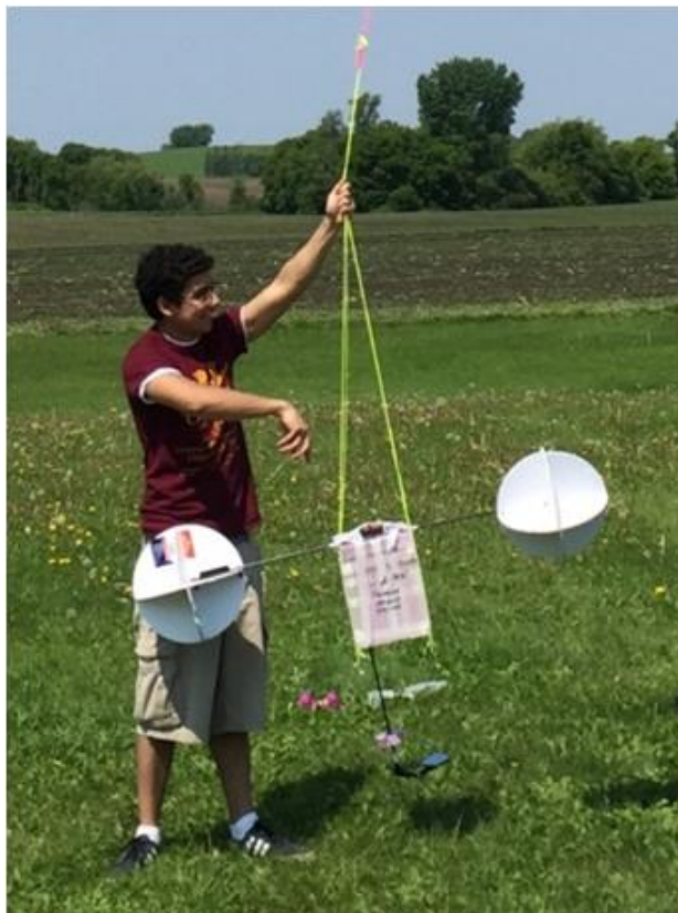
Fig. 3. U of MN student Victor Portillo prepares to release a single-payload balloon (parachute and 300-gram balloon are above, out of sight) with a 2-scoop "dumbbell" stabilizer. These two balls were attached to the ends of a single 1-m-long carbon fiber tube, so the device is significantly smaller than Rick Brennan's.
