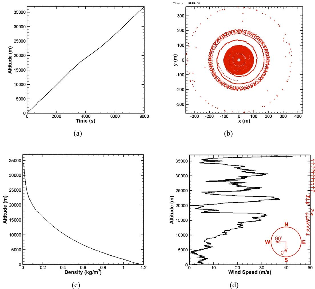
**Figure 1.** A sample set of weather data obtained at 00 UTC on 02-Jan-2013, including (a) the altitude of the meteorological balloon along time; (b) the relative position of the meteorological balloon to the observatory station, (c) air density, and (d) wind speed & direction along the altitude.
